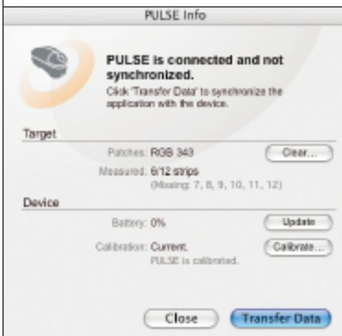
Connecting the X-Rite Pulse to the computer with the ColorElite software automatically opens the Pulse Info window. The top half indicates the missing rows (strips). The bottom half indicates battery charge and calibration status.
